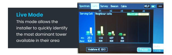
This allows the installer to focus on one specific operator at a time and find the dominant cell tower and its neighbours. Typically this mode will be used during the indoor testing to find the natural dominant tower. Then it can be used on the roof to locate this dominant tower. This helps in orientating the outdoor antenna correctly.
